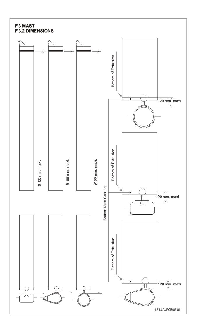
F.3 MAST **F.3.2 DIMENSIONS** MAST SPAR CIRCUMFERENCE 385 mm Maximum I.F18.A/PCB 01/01
